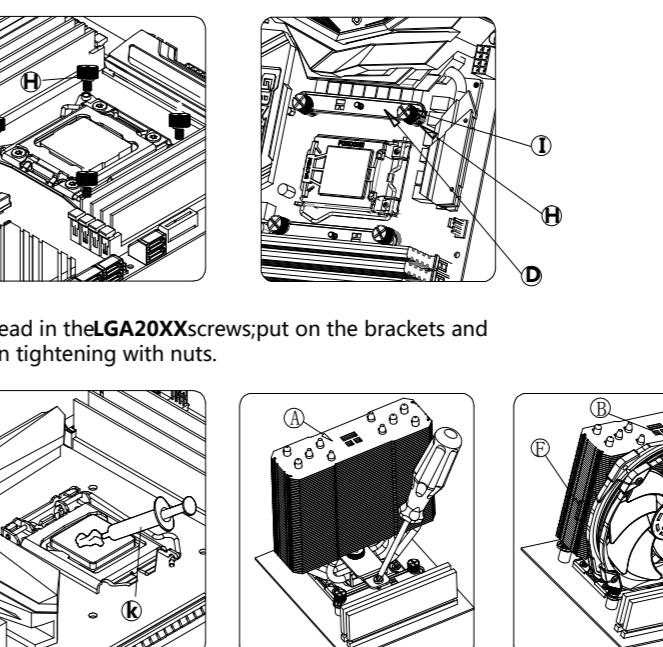
Thread in the LGA20XXscrews; put on the brackets and then tightening with nuts.
