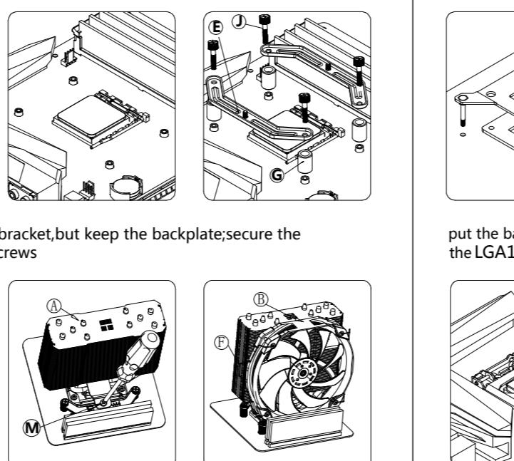
Remove plastic retention bracket, but keep the backplate; secure the brackets using the AM4 screws
