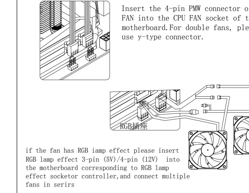
Insert the 4-pin PMW connector of the FAN into the CPU FAN socket of the motherboard. For double fans, please use y-type connector.
