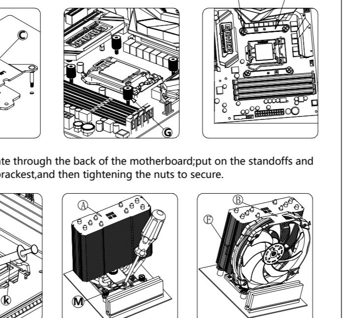
put the backplate through the back of the motherboard; put on the standoffs and the LGA115X bracket, and then tightening the nuts to secure.
