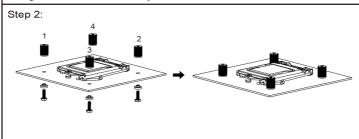
Step 2: Install the four screw pillars.
