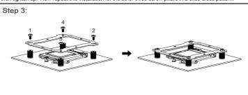
Step 3: Place the Anchoring Mount on the Screw Nuts.
