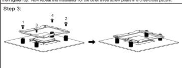
Step 3 : Place the Anchoring Mount on the Screw Nuts.
