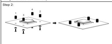
Step 2: Install the four screw pillars.
