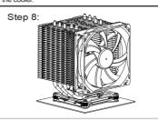
Step 8: Installation completed Plug in the fan connector to the CPU PWM Fan socket on the motherboard. Installation complete.
