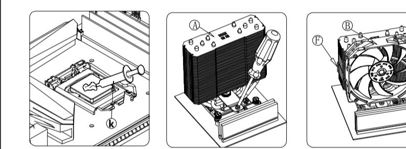
Apply a thin layer of thermal grease; and then secure heatsink.
