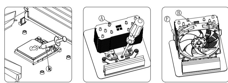
Apply a thin layer of thermak grease; and then secure heatsink.
