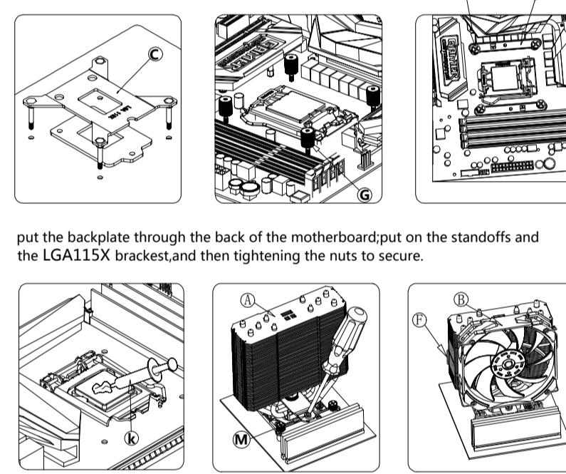
put the backplate through the back of the motherboard, put on the standoffs and the LGA115X bracket, and then tightening the nuts to secure.
