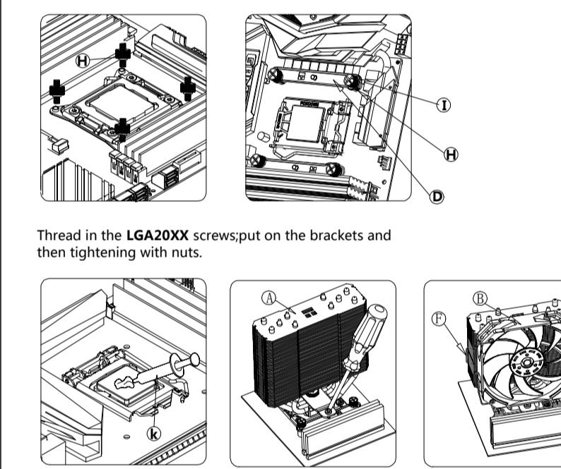
Thread in the LGA20XX screws; put on the brackets and then tightening with nuts.
