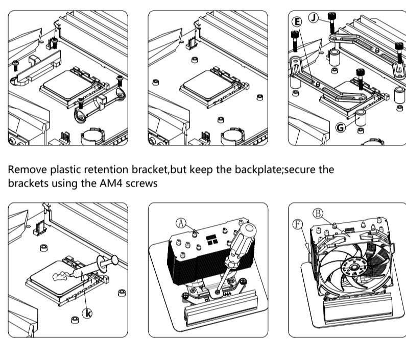
Remove plastic retention bracket, but keep the backplate; secure the brackets using the AM4 screws.
