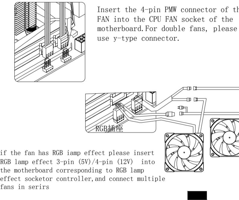
Insert the 4-pin PWM connector of the FAN into the CPU FAN socket of the motherboard. For double fans, please use y-type connector.
