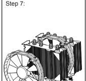
Step 7 : Place the 14x16cm fan onto the heatsink, and then secure it with the 14cm fan clips, plug in power.
